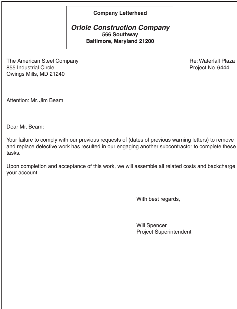
Letter 47 Engaging another subcontractor to correct defective work.
