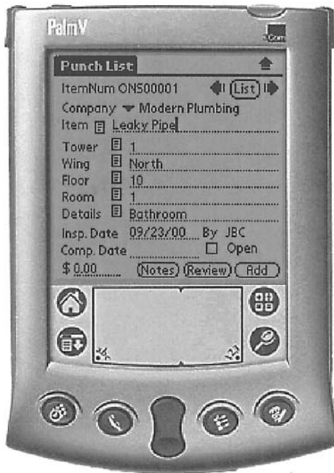
Figure 10-2 Screen shot of handheld computer with punch list software.
